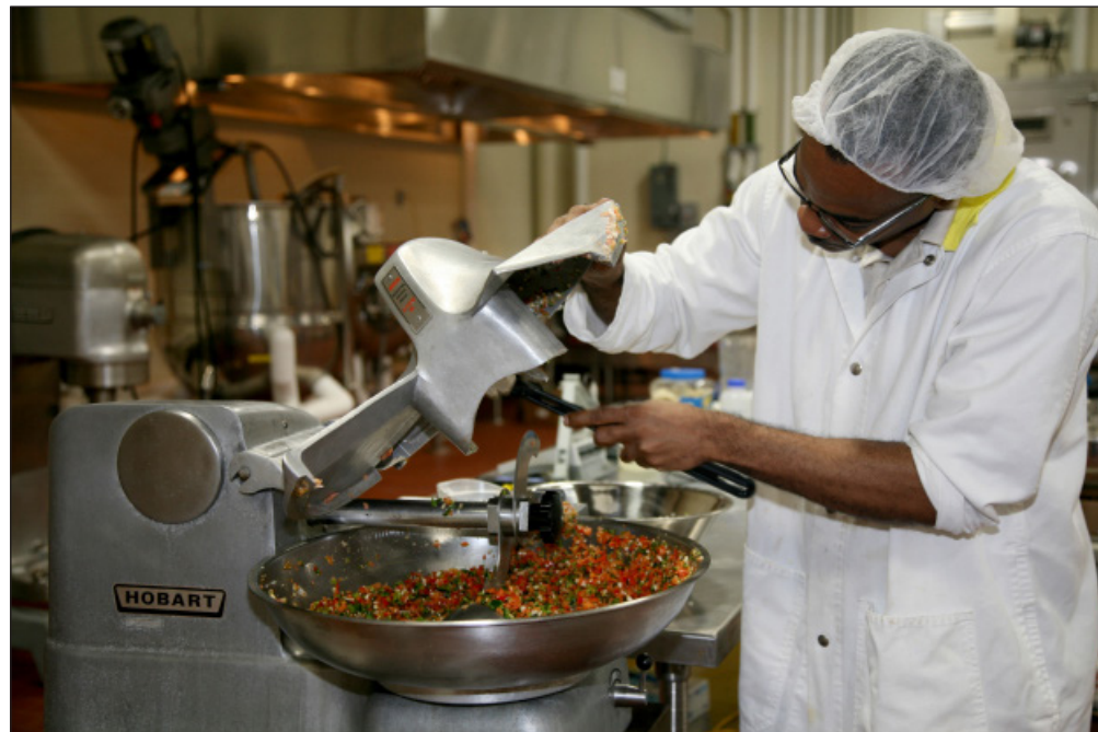
Darren Scott, FAPC food scientist and sensory specialist, uses a bowl chopper in the making of homemade salsa. FAPC photo
